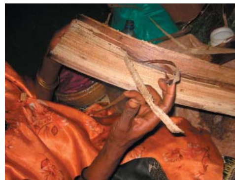
Peeling the inside layer of the fiber
